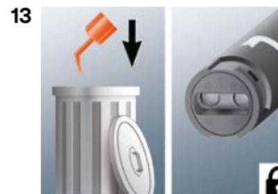
To unlock syringe fully rotate mixer until stop.
